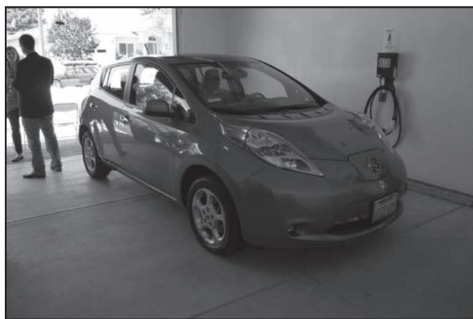
Figure 4. An electric vehicle, the Nissan Leaf, was included with the home. The garage was built with a charging station, as well as being pre-wired for an optional second charging station. Photo courtesy One Sky Homes.
