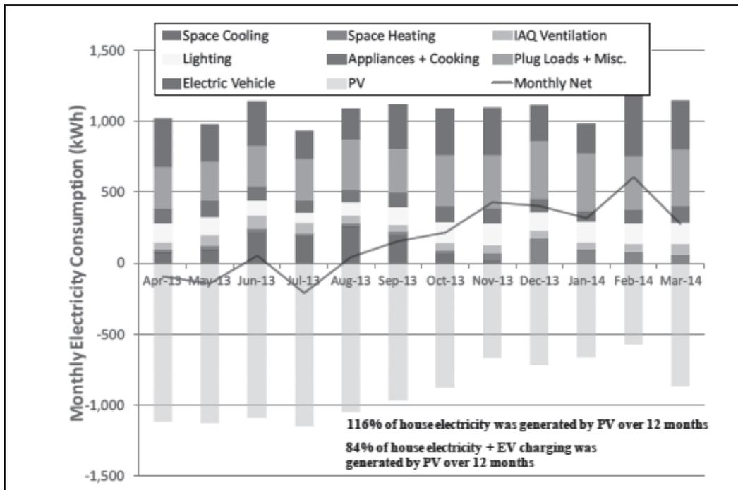
Figure 2. Monthly electricity consumption by end use and PV electricity generation (monthly net electricity shown as black line). Graphic courtesy Davis Energy Group, from *Cottle Zero Net Energy Home Monitoring Performance Evaluation Report, 12 Months Occupancy*, July 28, 2014.
