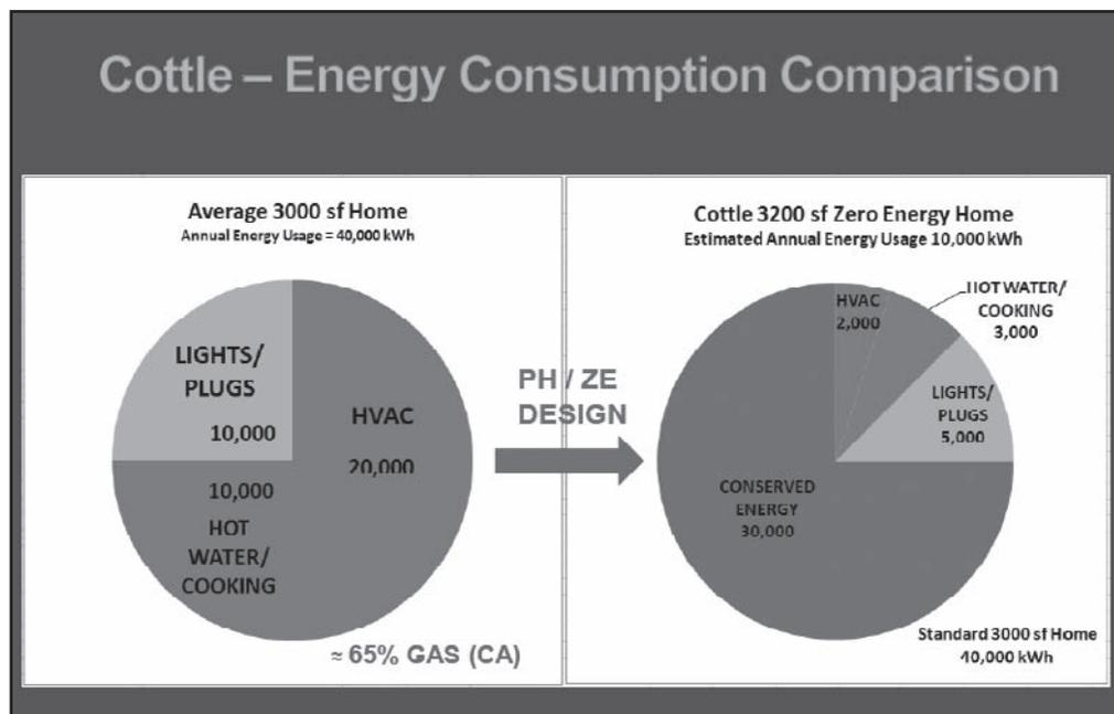
Figure 3. Energy consumption comparison. Figure courtesy Allen Gilliland and Davis Energy Group, from “Cottle Zero Energy Home” presentation.
